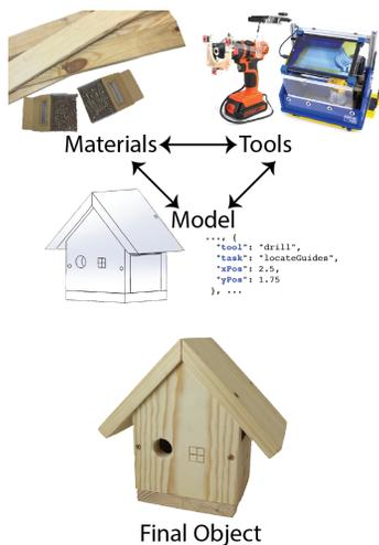
**Figure 1:** Drill Sergeant allows tools, materials, and model specifications to inform and define each other as a user works to create a final object.
