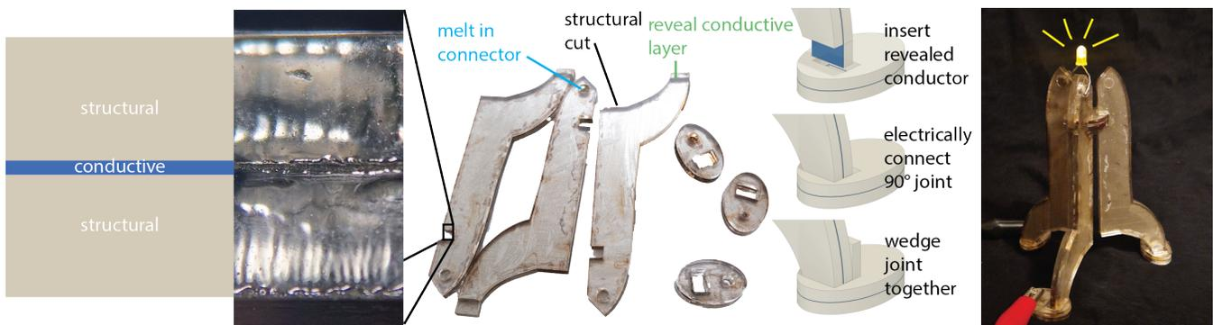
**Figure 1:** LaCir enables creating electrically-functional, structural objects on a laser cutter, through a laser-cutable substrate that features a conductive layer sandwiched between two structural layers (far left schematic, centre left photo) which can be cut in various ways (centre). We explore 3D joints to help conduct through connections (centre right) for fully-functional objects (right).
