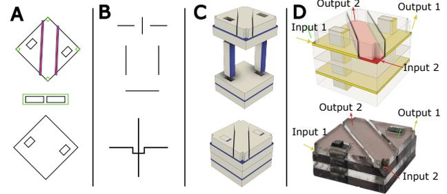
**Figure 13: A multilayer PCB, built from 4 individual pieces connected by laser-cut bridging joints. The SVG file has four parts: the top layer, two legs that bridge the layers, and the bottom layer (A). Before assembly, the parts create 6 separate circuits, but after assembly there are two independent coplanar connections (B). The pieces slide together vertically into a single assembly (C), which creates two independent input/output pairs from corner to corner (1 is yellow, 2 is red, D).**
