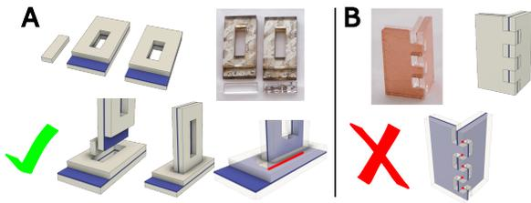
**Figure 3: Comparison of joints. A: a completely laser-cut joint to use with LaCir, which uses a revealing cut and a wedge for assembly. The red line highlights a line of possible connectivity. B: A traditional finger joint. Connectivity is only made on the intersecting points between each of the fingers. This is highlighted with the red dots in the rendered picture.**
