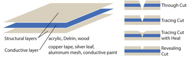
**Figure 2: The LaCir substrate is composed of two structural layers sandwiching a conductive layer (left), and we tried various materials for each (left, bottom). We present four cuts to manipulate LaCir substrates (right): through cuts, tracing cuts, tracing cuts with heal, and revealing cuts.**
