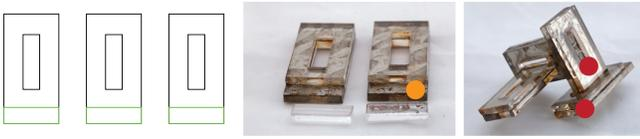
Figure 7: For our conductive layer tests, we cut objects of fixed geometry (left) with varying conductive layers. We clipped them to an ItsyBitsy at the orange point and attempted to use the CapTouch library (centre). We then measured resistance across single parts, and through 1 and 2 joints at, e.g., the two joints between the red points (right).
