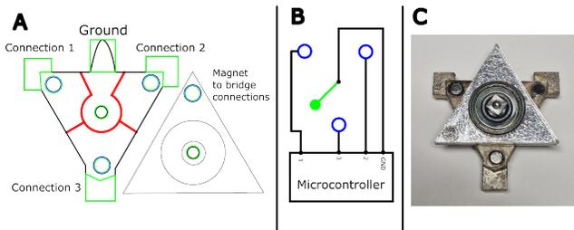
**Figure 12: A wheel of fortune example application created with LaCir, comprised of individual pieces connected using ball bearings, screw inserts and magnets. The cut schematic shows tracing cuts (red) that separate the segments, and a donut-shaped cutout for the press-fit ball bearing insert (A). The circuit diagram highlights the top layer (green) that spins with a magnet on the end, connecting to one of three endpoints (blue) (B). This is visible in the fully assembled device (C).**
