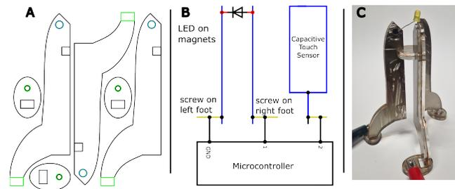
Figure 11: A lamp shaped like a rocketship, built from 6 individual pieces (A) connected by laser-cut joints and connectors. The lamp's circuit connects the micro-controller through two feet via healed-in screw inserts (yellow), up through the legs (blue), and to the LED with magnets (red) (B). The third foot and leg are configured as a capacitive touch sensor. Assembling and connecting the lamp lights it up (C).
