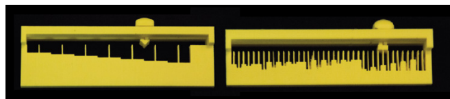
Figure 3. We experimented with two different encoding mechanisms for sliders: linearly increasing sequences (left) and de Bruijn (right). de Bruijn sequences allow classification of fewer tine lengths, but require more consecutive tine recognitions to determine position and direction.
