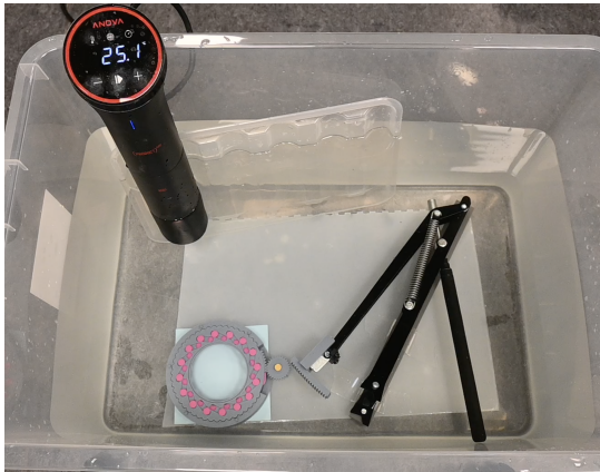
Figure 9: Setup for evaluating System 2 end-to-end and testing temperature sensitivity
