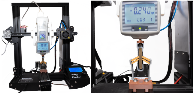
Figure 10: Our force-displacement test rig is built on a modified Creality Ender 3 Pro 3D printer and an off-the-shelf push/pull force meter.
