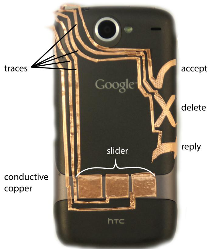
Figure 1.2: A Midas-generated interface with buttons for checking email mounted on the back of a smart phone.
