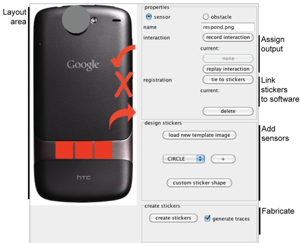
Figure 4.2: Midas’s sensor editor takes its cues from GUI editors: designers first lay out sensing areas through direct manipulation; they later define interactions for each sensor using a property inspector.
